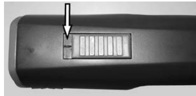
Fig. 5 Switch in ON-position ("I")
