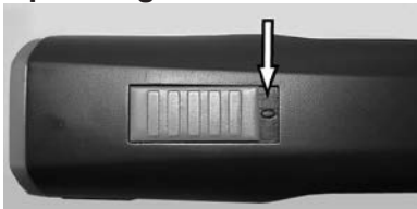
Fig. 4 Switch in OFF-position ("0")
